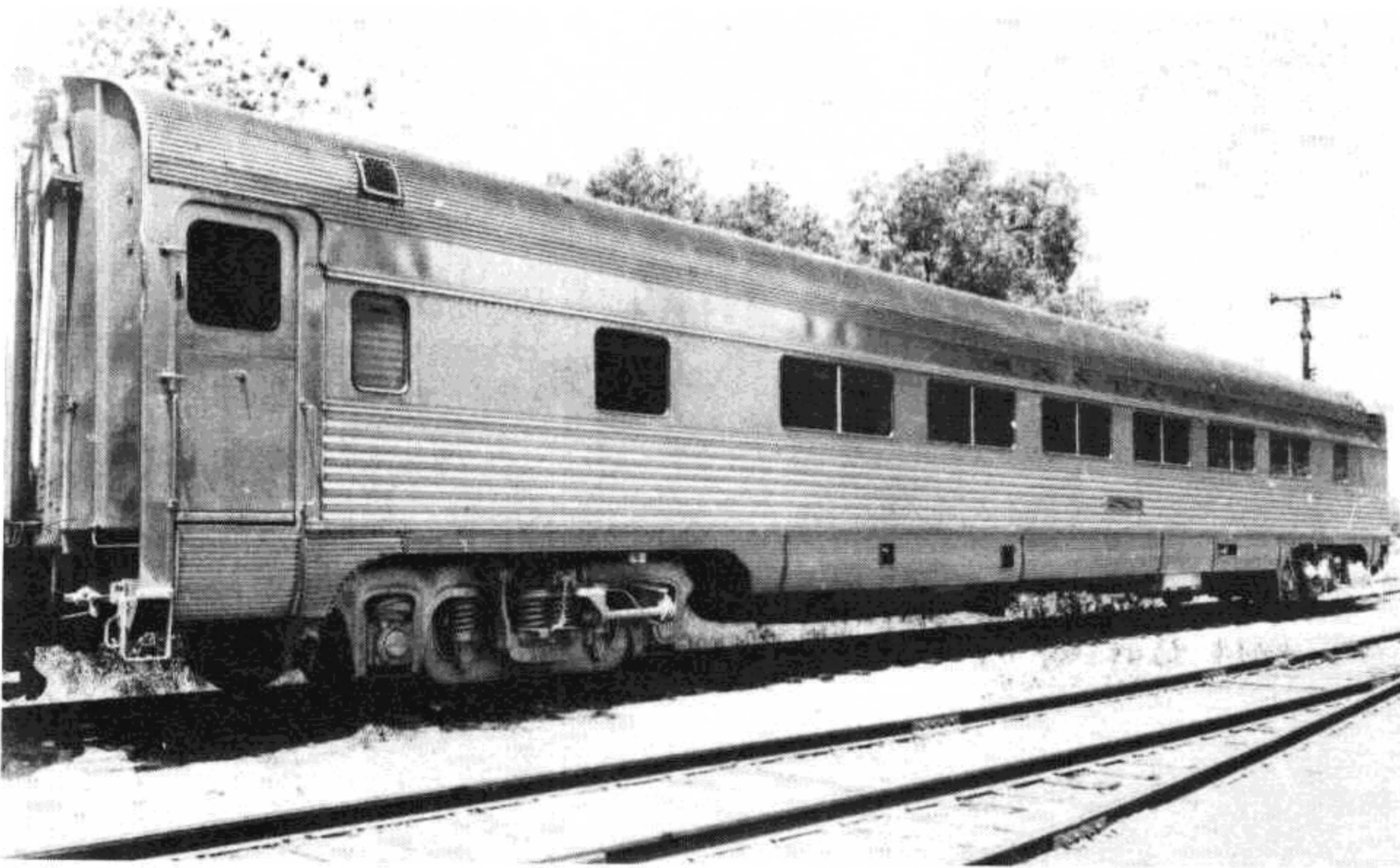
Budd fluting of the 1953-1964 period on Chair Car No. 2823. Roof fluting immediately identifies this as a Budd car. Photo by Dennis Kogan.
